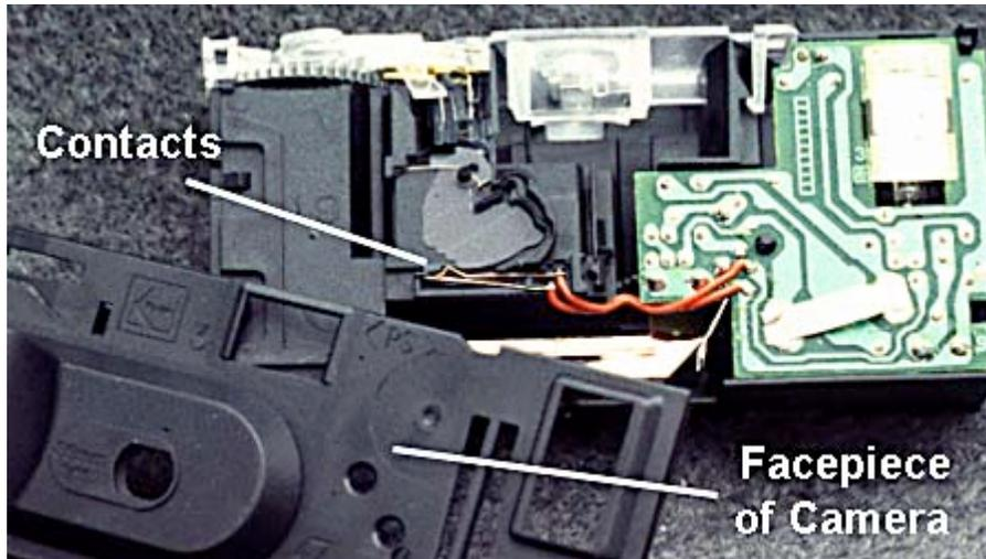
2. The flash contacts are two long, thin copper pieces below the lens aperture. They are attached to red wires. Using a screwdriver with an insulated handle, short across the contacts. If the flash capacitor is charged, this will discharge it. Be prepared for a flash of light, just in case. Now you can cut the copper contacts from the wires. Leave as long a length of wire as possible. Strip both wires about a quarter of an inch.
