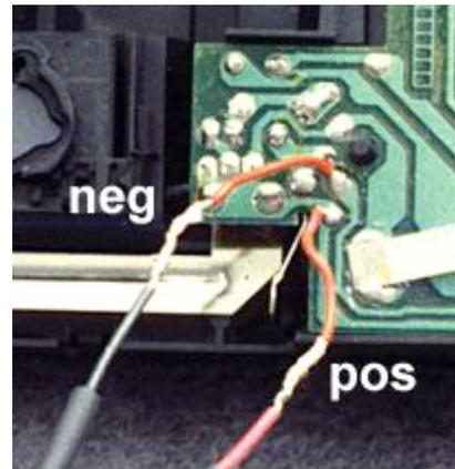
4. Twist the positive leads together and solder them. Repeat with the negative leads. Wrap each splice with electrical tape or use heat shrink tubing. Then you can reassemble the camera. A photograph is shown below.
