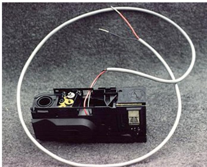
5. Before connecting the sound trigger, test the flash as follows. Put a battery in the battery compartment of the camera. Charge the flash using the button below the flash. You'll hear a high-pitched whine as the unit is charging. An orange light will blink when the flash is ready, and you can release the button. Now short the two wires together, being sure not to touch the bare leads. If your connections inside the camera are secure, the flash should discharge.
