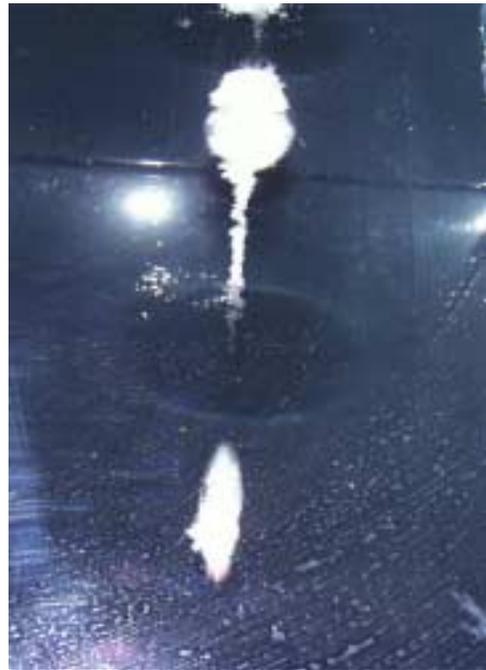
This image was taken at a later point in the water entry, and the cavity left has separated in the middle. Less blurring in this image is likely the result of slower speeds.
