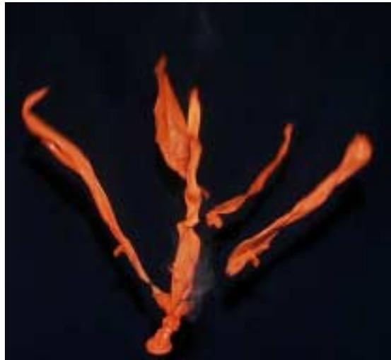
This photo was taken much later in the burst than the photo to the left. The balloon has completely ripped into fragments.
